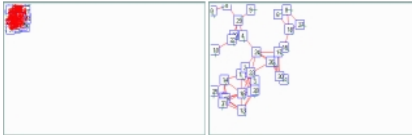
Fig 3. Initial robot deployment Fig 4. Robot distribution after 40 timesteps
